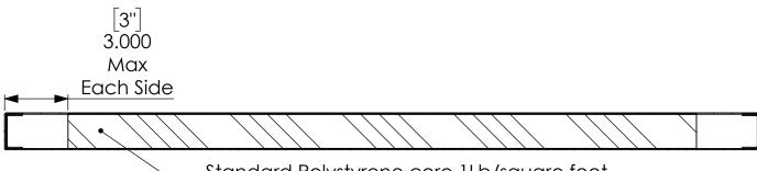
Standard Polystyrene core 1Lb/square foot Other polystyrene core densities avaliable
