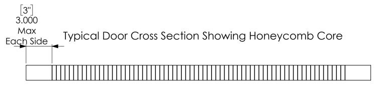
Vertical Paper Honeycomb 1/2" 60-60-15% Attached using glue in specs
